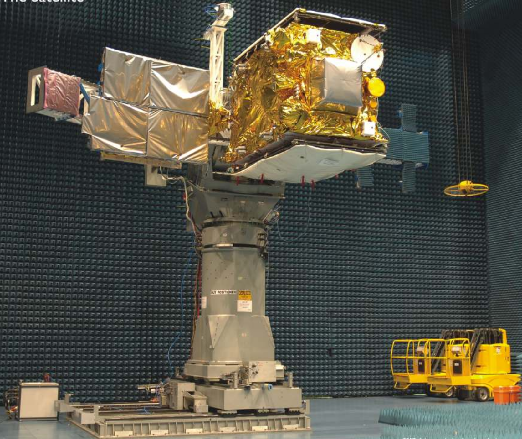
GSAT-4 in anechoic chamber during one of the prelaunch tests
