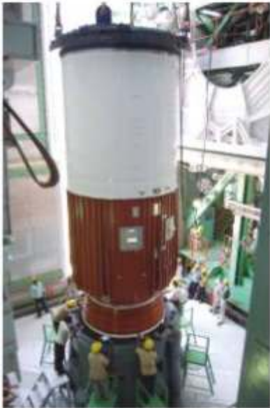
Positioning of nozzle end segment of PSLV-C14 first stage
