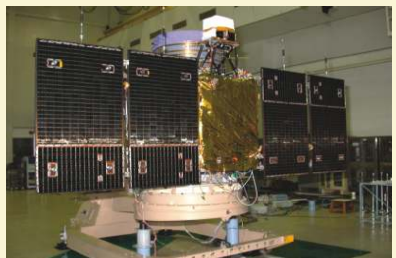
CARTOSAT-2B SATELLITE IN CLEAN ROOM WITH ITS PANELS DEPLOYED
