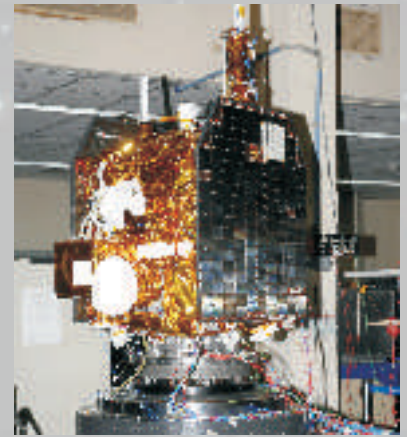
Youthsat undergoing vibration test at ISRO Satellite Centre
